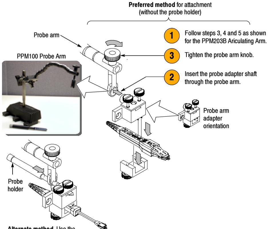
**Alternate method.** Use the probe holder provide with the PPM100 Probe Arm.
